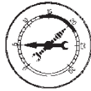
BLOWN HEAD GASKET AT IDLE
