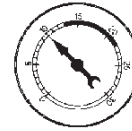
LATE VALVE TIMING, VACUUM LEAK AT IDLE
