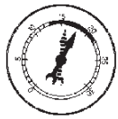
POOR VALVE SEATING AT IDLE
