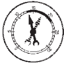
STICKING VALVE AT IDLE
