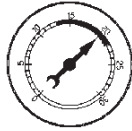
NORMAL READING RANGE AT IDLE
