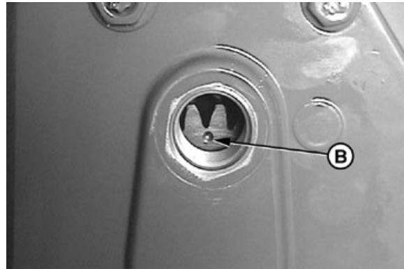
High pressure pump gear timing mark
