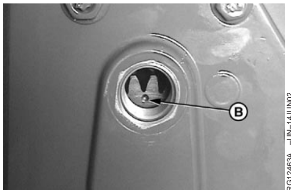
High pressure pump gear timing mark
