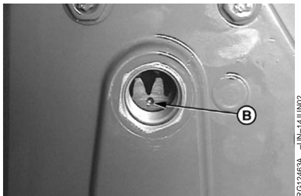
High pressure pump gear timing mark
