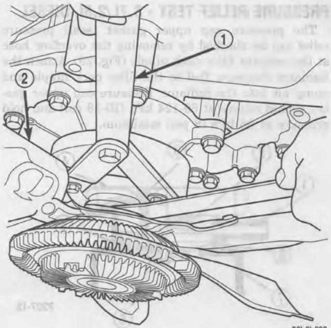
**Fig. 31 Viscous Fan and Fan Drive 3.7L**
