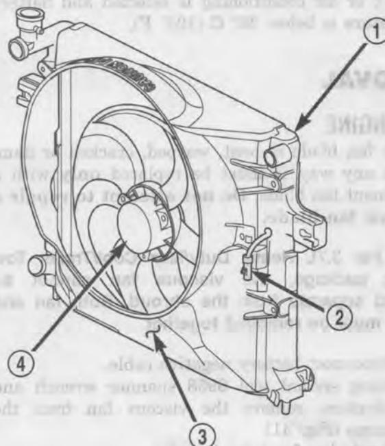
**Fig. 30 Radiator Cooling Fan - Typical**
