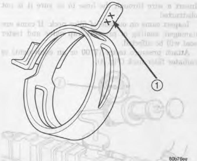
**Fig. 2 Spring Clamp Size Location**
