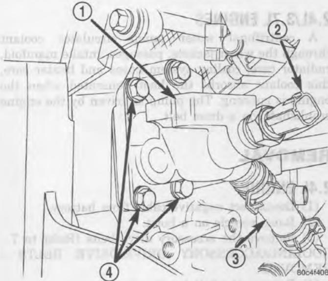
**Fig. 39 Thermostat Housing**
