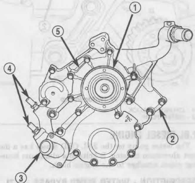
**Fig. 40 Water Pump and Timing Chain Cover**
