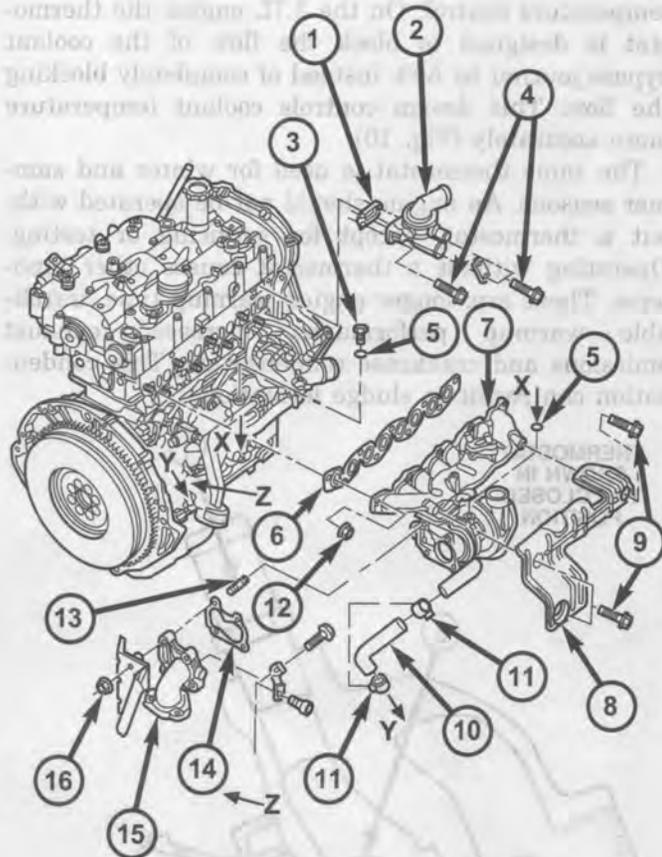
Fig. 11 THERMOSTAT HOUSING
