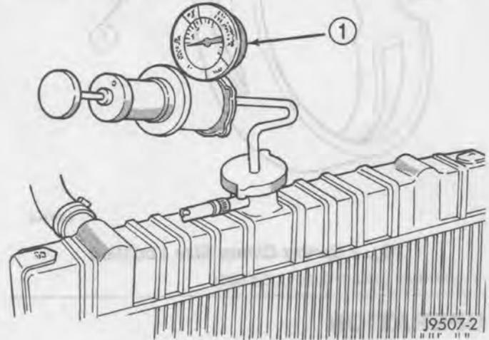
**Fig. 4 Pressure Testing Cooling System - Typical**
