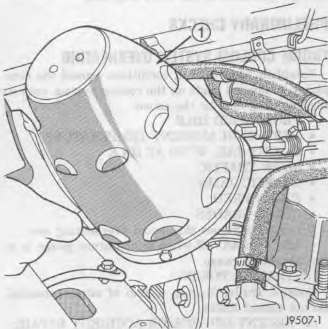
**Fig. 3 Leak Detection Using Black Light - Typical**
