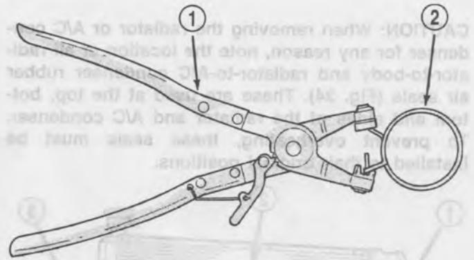
**Fig. 22 Hose Clamp Tool - Typical**
