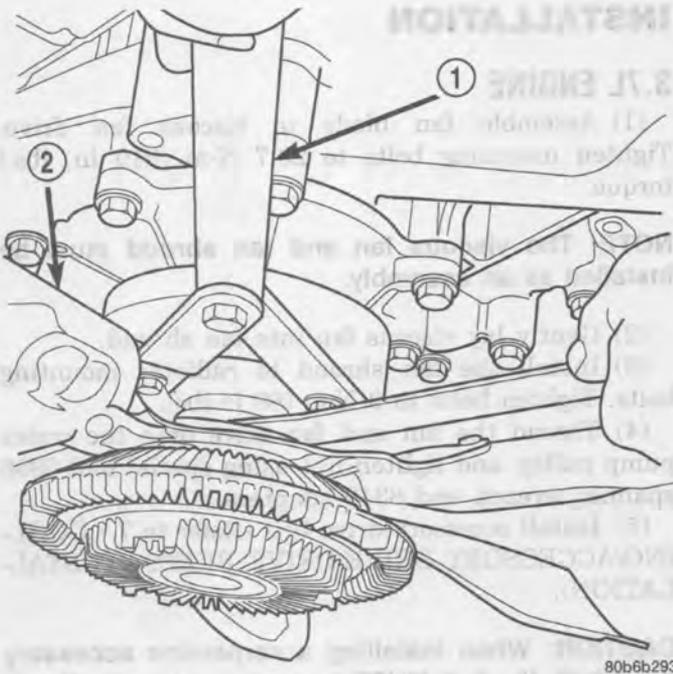
**Fig. 35 Viscous Fan and Fan Drive 3.7L**
