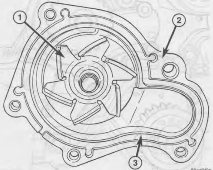
**Fig. 46 Water Pump Body**
