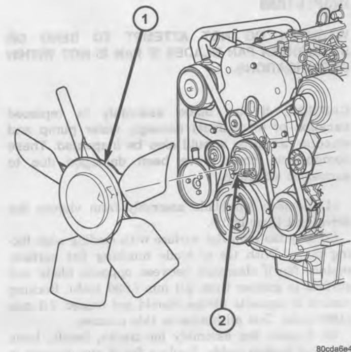
**Fig. 37 COOLING FAN AND VISCOUS CLUTCH**
