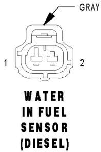
**WATER IN FUEL SENSOR (DIESEL) - GRAY 2 WAY**
