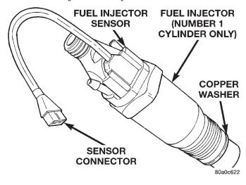
Fig. 23 Fuel Injector Sensor Location
