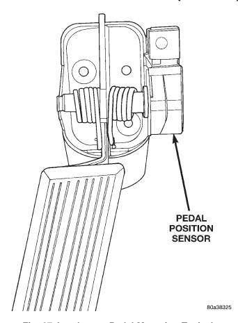
Fig. 27 Accelerator Pedal Mounting-Typical
