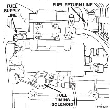
Fig. 11 Fuel Timing Solenoid
