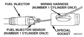
Fig. 43 Wiring Harness Through Socket
