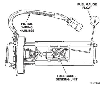
Fig. 31 Fuel Level Sensor
