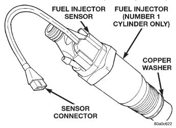
Fig. 17 Fuel Injector Sensor
