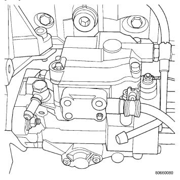
Fig. 5 Fuel Injection Pump
