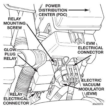
Fig. 30 Power Distribution Center (PDC) Location FUEL LEVEL SENSOR
