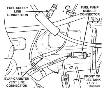
Fig. 44 Fuel Tank Connections at Front of Tank
