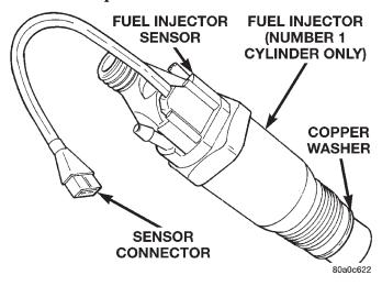
Fig. 41 Fuel Injector Sensor—Number-1 Cylinder
