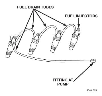
Fig. 9 Fuel Drain Tubes
