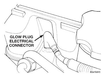
Fig. 17 Wiring Connection at Glow Plug
