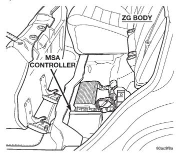
Fig. 1 MSA Controller Location
