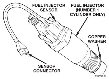
Fig. 7 Fuel Injector Sensor
