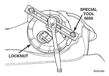
Fig. 47 Fuel Reservoir Module Lock Nut Removal
