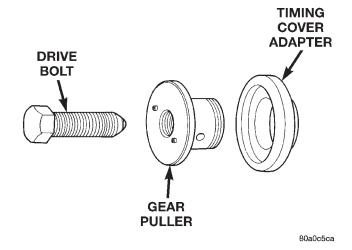
Fig. 36 Pump Gear Tools
