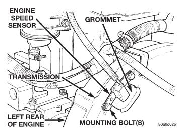
Fig. 19 Engine Speed Sensor
