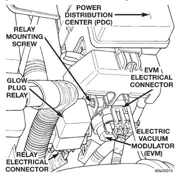
Fig. 23 Glow Plug Relay Location
