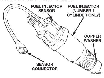
Fig. 3 Fuel Injector Sensor
