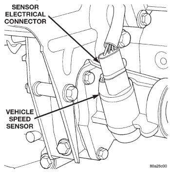
Fig. 8 Vehicle Speed Sensor—Typical
