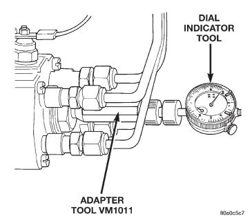
Fig. 40 Installing Dial Indicator and Special Adapter
