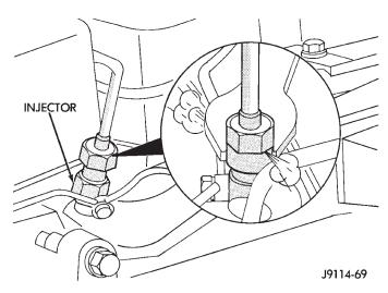
Fig. 26 Bleeding High-Pressure Fuel Line—Typical
