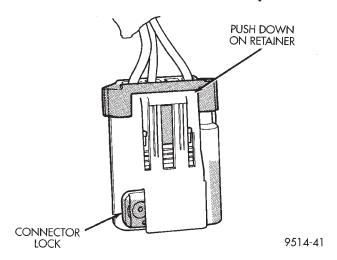
Fig. 46 Module Connector Retainer and Lock
