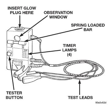
Fig. 15 Typical Glow Plug Tester
