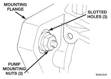
Fig. 38 Injection Pump Mounting Nuts
