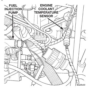
Fig. 14 Engine Coolant Temperature Sensor Location
