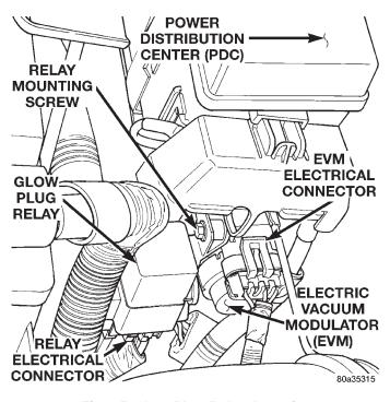
Fig. 15 Glow Plug Relay Location
