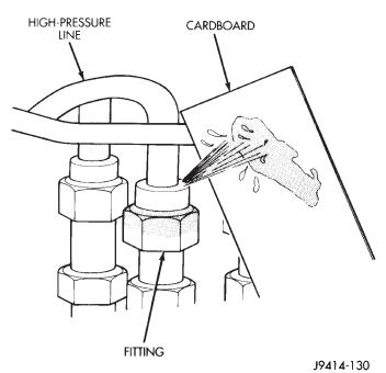
Fig. 24 Typical Test for Leaks with Cardboard
