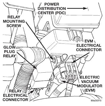
Fig. 12 Glow Plug Relay Location
