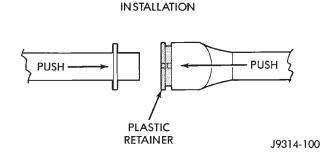
Fig. 8 Plastic Retainer Ring-Type Fitting
