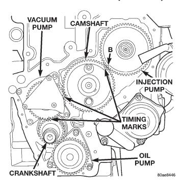
Fig. 21 Vaccum Pump at Front of Engine
