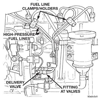
Fig. 48 Fuel Lines and Clamps/Holders
