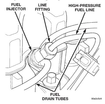
Fig. 42 Fuel Injector—Typical
