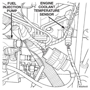
Fig. 20 Engine Coolant Temperature Sensor Location
