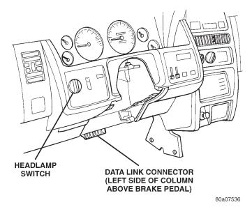
Fig. 7 Data Link Connector Location
