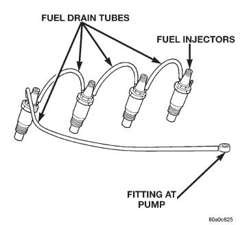
Fig. 28 Fuel Drain Tubes
