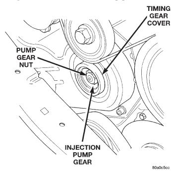
Fig. 35 Removing Pump Drive Gear Nut
