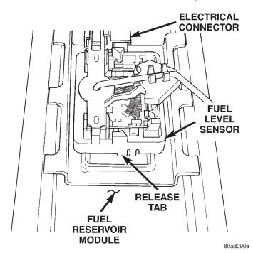
Fig. 32 Fuel Level Sensor Release Tab
