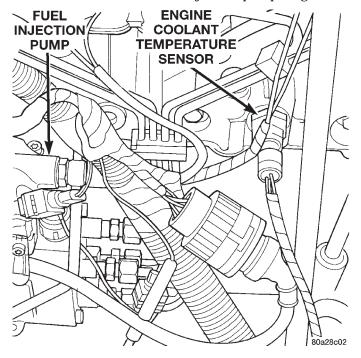
Fig. 4 Engine Coolant Temperature Sensor Location
