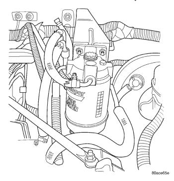
Fig. 3 Fuel Filter/Water Separator Location
