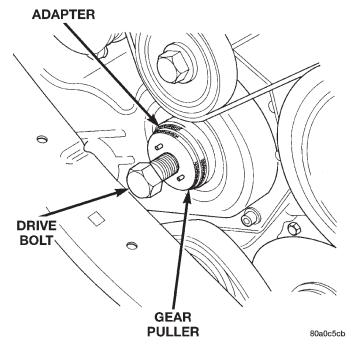
Fig. 37 Installing Pump Drive Gear Removal Tools
