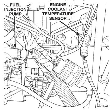
Fig. 20 Engine Coolant Temperature Sensor Location
