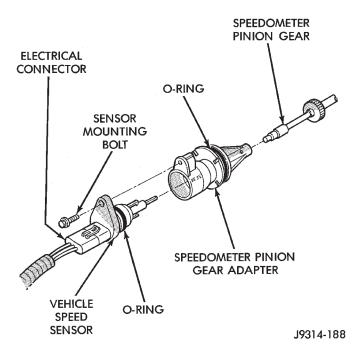
Fig. 27 Sensor Removal/Installation—Typical INSTALLATION
