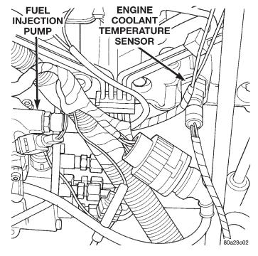
Fig. 34 Engine Coolant Temperature Sensor
