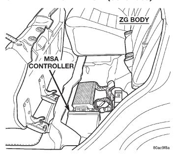
Fig. 2 MSA Controller Location
