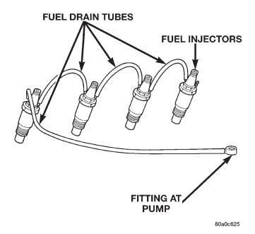
Fig. 6 Fuel Injectors and Drain Tubes
