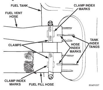
Fig. 45 Fuel Fill/Vent Hose Index Marks
