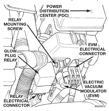
Fig. 16 Glow Plug Relay Location
