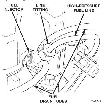
Fig. 49 Fuel Lines at Fuel Injectors
