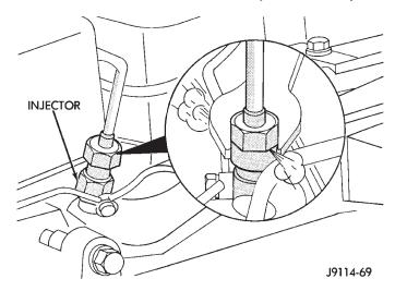
Fig. 22 Typical Inspection of Fuel Injector
