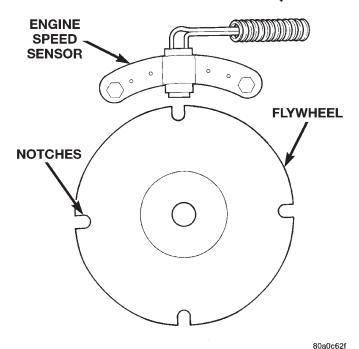
Fig. 6 Speed Sensor Operation
