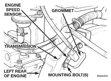
Fig. 5 Engine Speed Sensor Location
